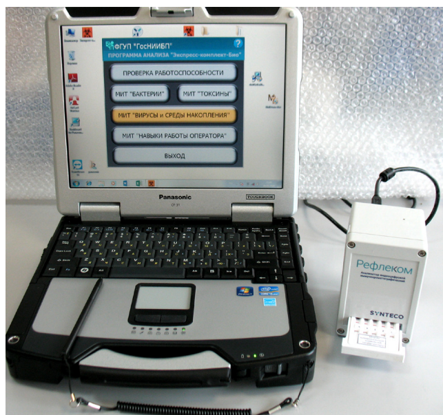
Fig. 3. Exterior view of the reflectometer device of EkB kit
